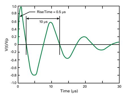
The 100 kHz Ring Wave (voltage and current)
