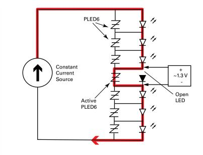
Figure 15. PLEDs protect series wired LED strings should one fail as an open circuit, the most common failure mode.
