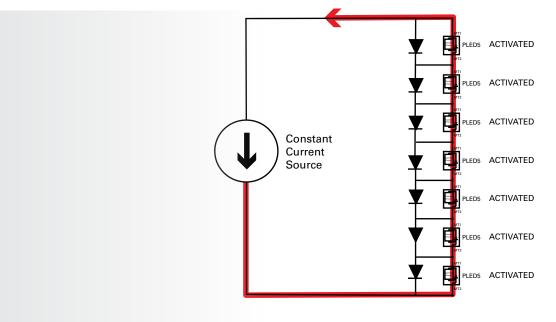
Figure 16. PLEDs also protect LED strings from reverse polarity situations.
