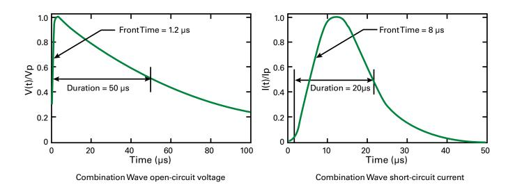
Figure 4. IEC 61000-4-5 surge immunity test waveforms: 1.2×50µs open circuit voltage and 8×20µs short circuit current.
