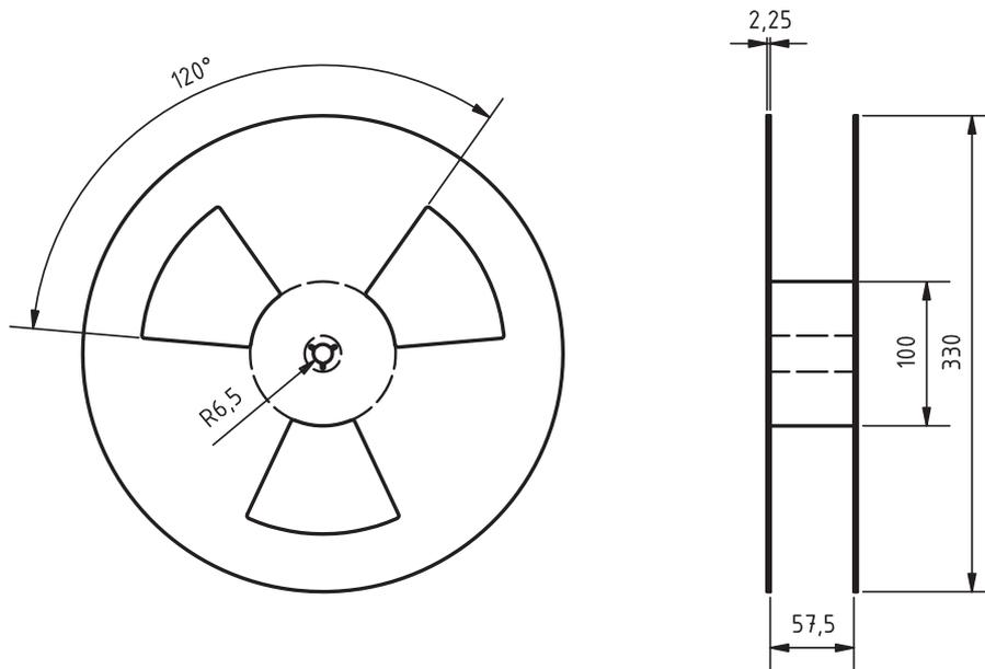
Fig. 6 Dimensions of the Reel
