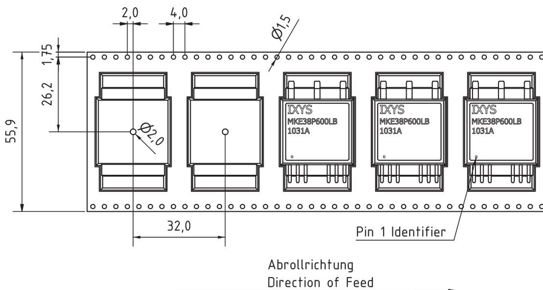
Fig. 5 Dimensions of the Tape
