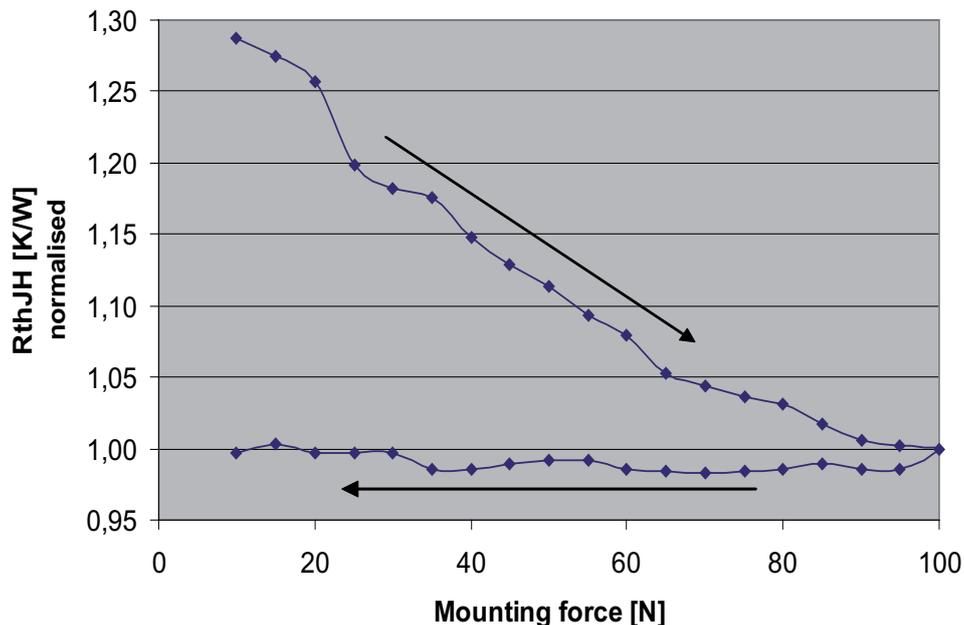
Fig. 9 Change of the thermal resistance junction to heat sink ( $R_{thJH}$ ) versus mounting force
