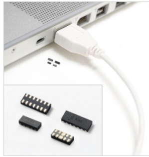
Fig. 6: Littelfuse SP3012-04UTG and SP3012-06UTG TVS Diode Arrays were specifically designed for USB 3.0 protection.
