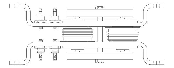
The PPI-600V is a ground-wire device that allows a trailing-cable ground to be monitored independently of the parallel ground path created when trailing-cable-fed equipment is in contact with the earth. It also allows a trailing-cable ground to be monitored in the presence of stray dc and it prevents inter-machine arcing caused by the voltages induced in the cables.
