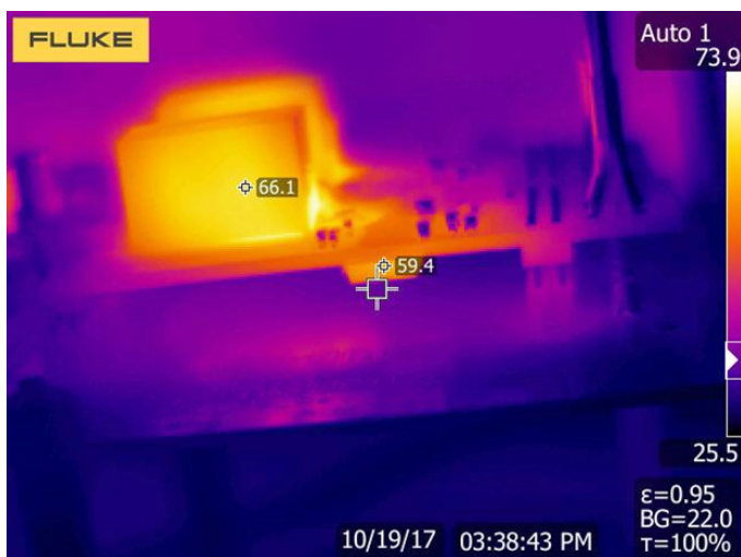
Figure 18: Thermal image of the LSICRD-GD-ISO5852 with ISO5852S and 2 Ohm gate resistance operating at 100 kHz
