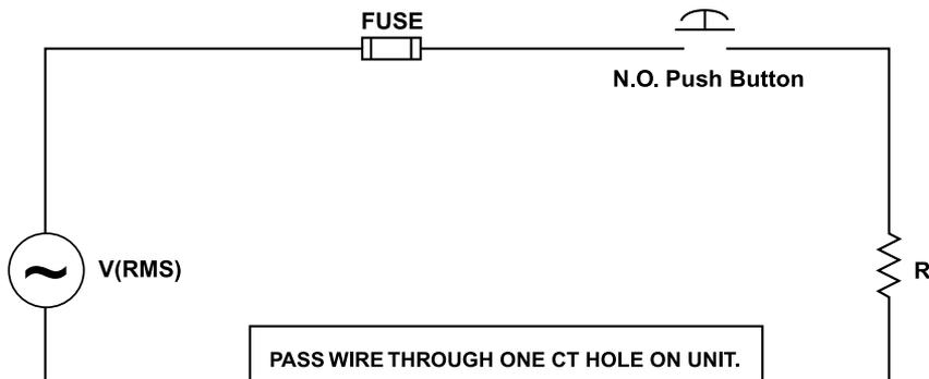
5. The values of V and R will be determined by the current required to generate a GF trip condition:  $I = V_{rms}/R$ , where I = 115% of GF setting.
